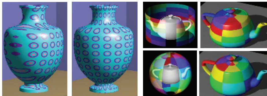
Figure 14.12. This figure shows orthogonal (left) and cylindrical (right) mapping on a vase and a cylindrical mapping (top) and a spherical mapping (bottom) on a teapot.
