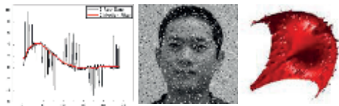
Figure 1.14. This shows the outliers or salt and pepper noise in 1D (left), 2D (middle) and 3D (right) data. On the left, we show the effect of a median filter in removing the outliers in red.
